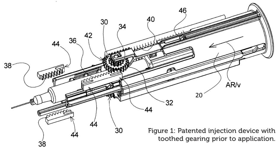
Figure 1: Patented injection device with toothed gearing prior to application.
