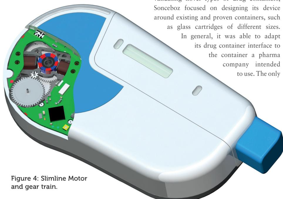
Figure 4: Slimline Motor and gear train.
