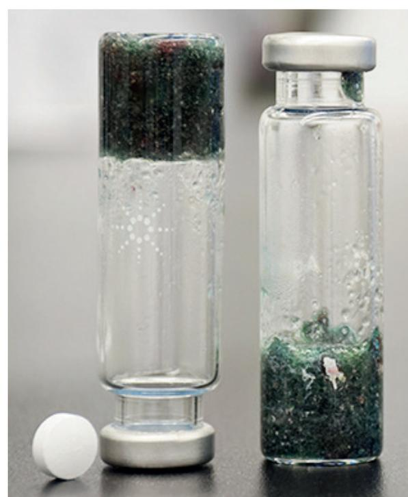
Figure 4: The hard, coloured gel that forms immediately when Intellitab<sup>™</sup> tablets are ground and added to liquids.
