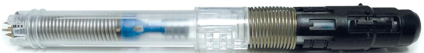
**Figure 2:** Most autoinjectors are driven by a delicate balance between a main spring and a return spring.
