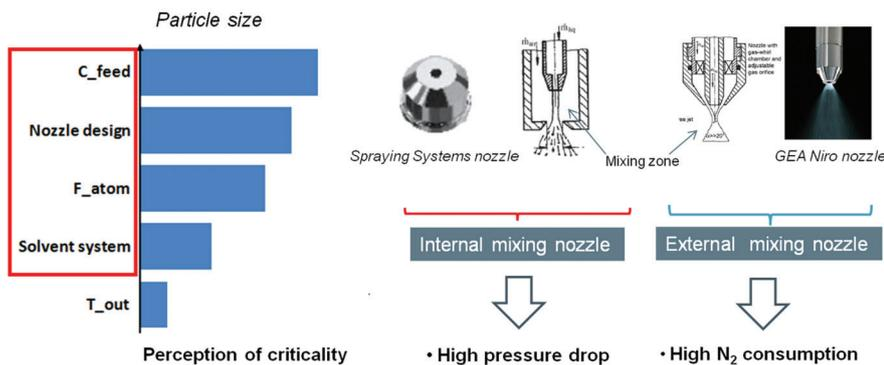
Figure 4: Main critical parameters and challenges during the atomisation step.  $C_{feed}$  = solids feed concentration,  $F_{atom}$  = flowrate of atomisation gas, and  $T_{out}$  = outlet drying gas temperature (Nozzle schemes adapted from Hede et al, 2008.)
