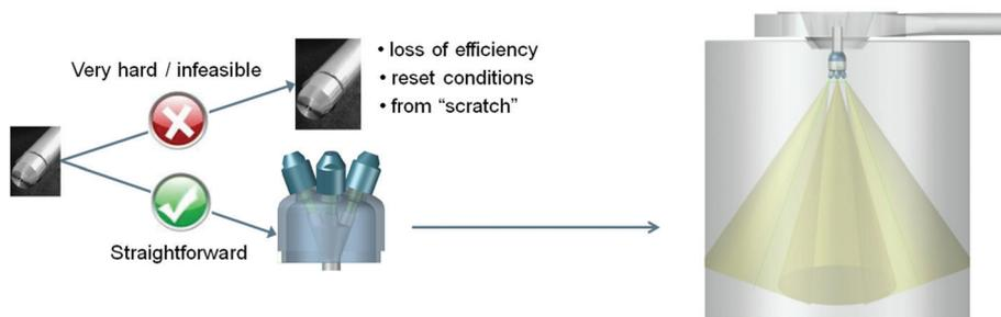
Figure 5: Multi-nozzle approach for expediting scale-up of atomisation (Hovione's apparatus).<sup>12</sup>
