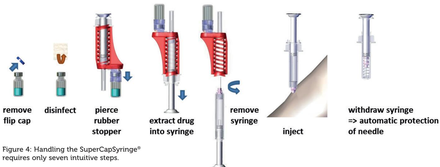
Figure 4: Handling the SuperCapSyringe® requires only seven intuitive steps.
