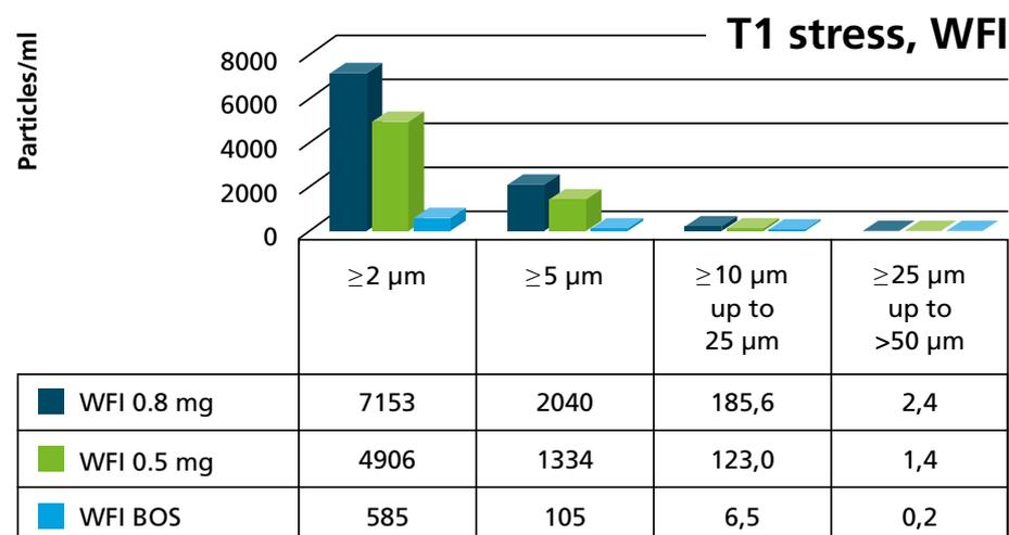
Figure 4: Sub visible silicone oil particles ≥ 2 µm WFI solution.
