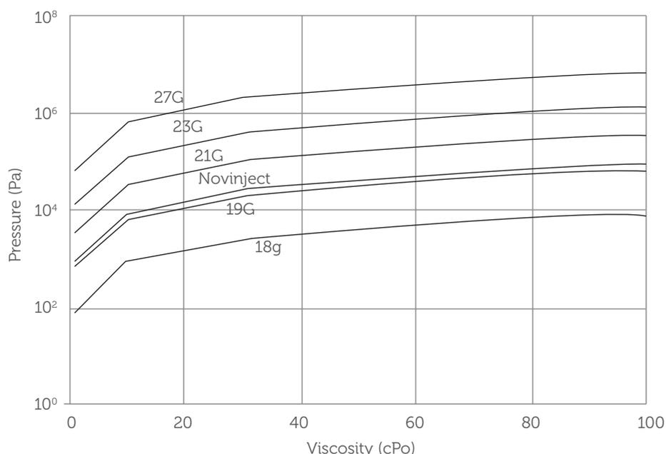
Figure 3: Theoretical pressure for different needle gauges and Novinject microneedles to inject 1 mL/min of solution.
