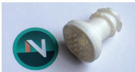
Figure 4: Possible Luer configuration for the microneedle array.
