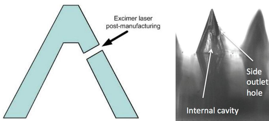
Figure 2: Original design of Novinject microneedle solutions.
