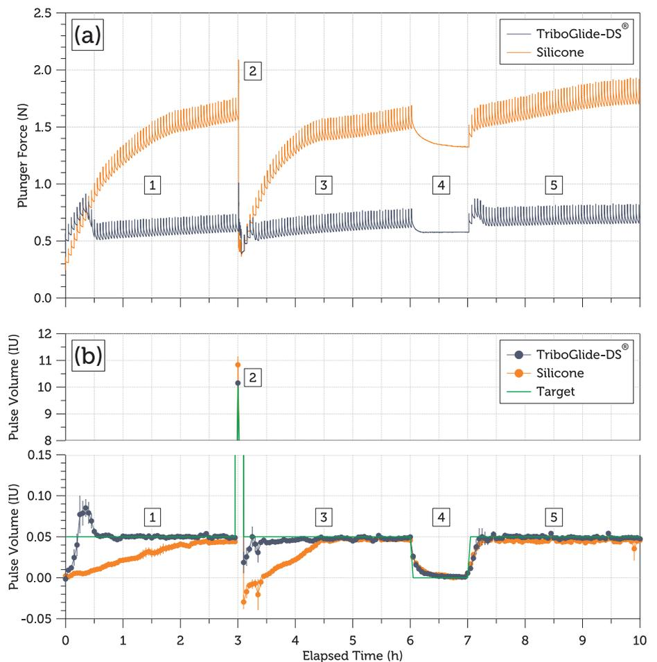
Figure 4: (a) Plunger force versus test time and (b) individual pulse volume versus test time for the realistic pump profile. The five different pump regions are labelled on the plot where [1, 3, and 5] correspond to basal delivery, [2] is a mealtime bolus and [4] is a pump shut-off.
