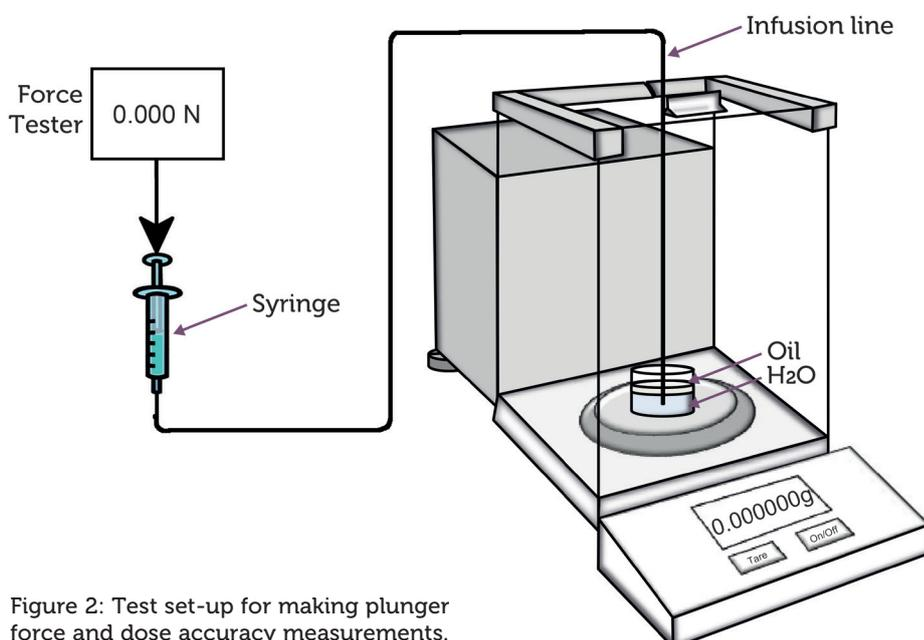
Figure 2: Test set-up for making plunger force and dose accuracy measurements.
