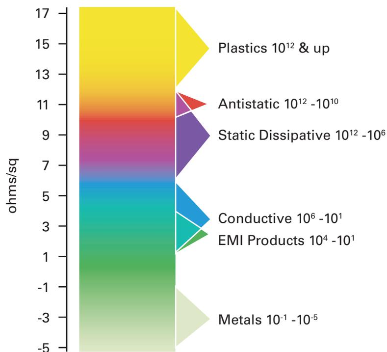
Figure 1: Surface resistivity spectrum for conductive materials.
