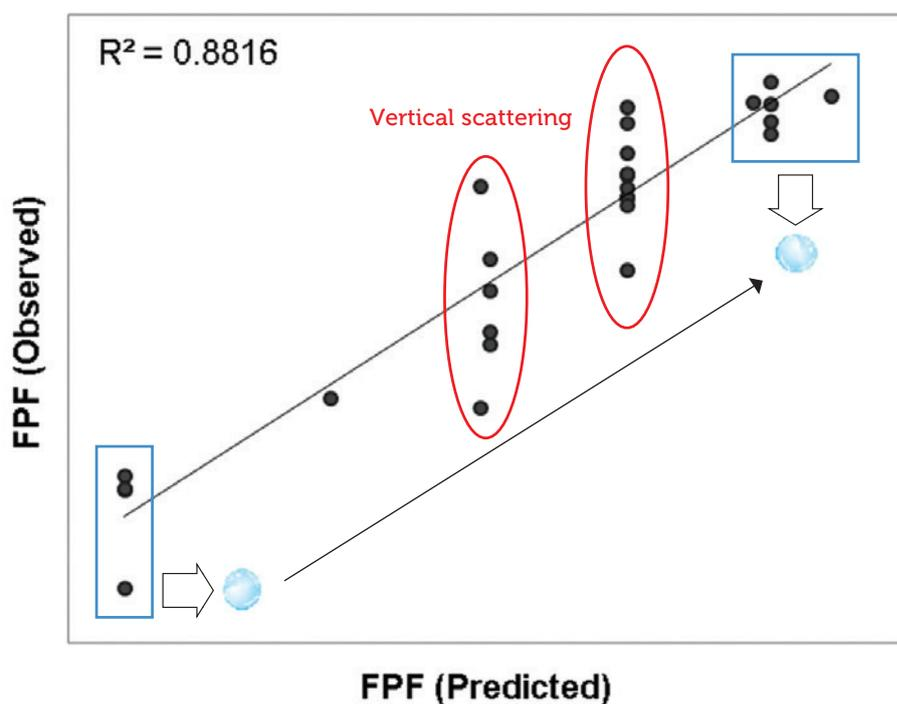
Figure 5: Statistical model for FPF with SD feed droplet related parameters as input factors. The in vitro aerodynamic performance was determined using a modified gravimetric Andersen cascade impactor.
