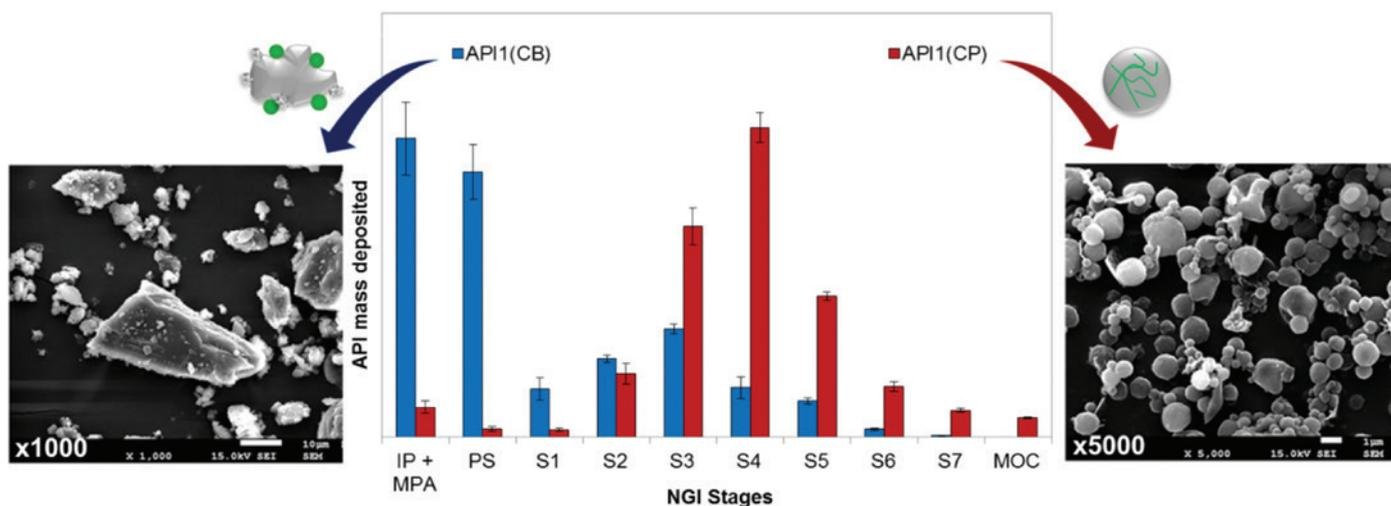
Figure 9: Aerodynamic performance of the CB (carrier based) and CP powder formulated with API model drug 1 (API1) by an NGI with chemical recovery at 60 L/min using a Plastiapre HR device model 7 operated at 4 kPa, where MPA, IP, PS, S1 and MOC stands for Mouthpiece adaptor, induction port, pre-separator, stage 1 and micro-orifice collector respectively.
