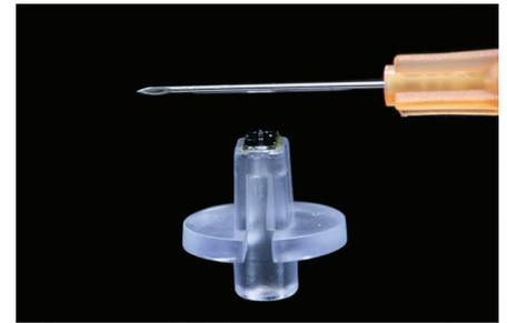
Figure 5: Comparison between a microneedle and a 25G needle.
