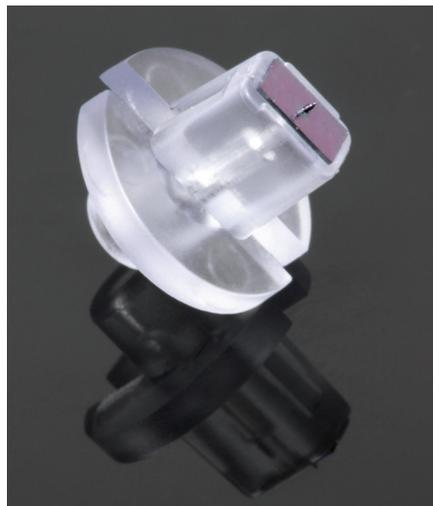
Figure 2: Single microneedle mounted on a connector.
