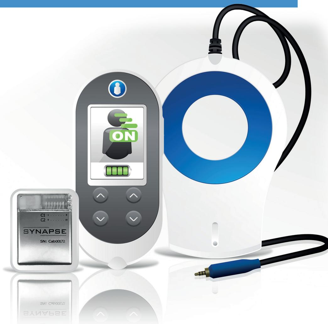
Figure 2: Nexeon's Synapse deep brain neurostimulation system includes: leads implanted into the deep part of the brain (front); implantable pulse generator typically implanted in the subclavicular region (left); patient controller (center); external battery recharger (right); and the physician reprogrammer tablet (rear).
