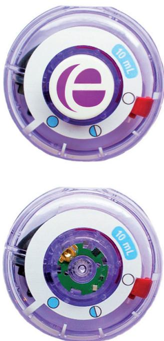
Figure 1: The Enable Smart Device with the button cover in place (top) and the button cover removed showing the chip (bottom).
