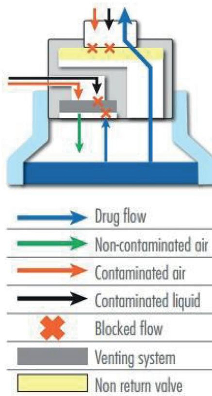
**Figure 3: The Novelia® system uses a non-return valve that removes the need to filter the liquid. This makes it possible to use a silicone membrane to filter the air.**
