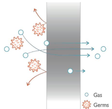
**Figure 4: The PureFlow™ technology consists of using the air permeation property of the silicone to allow the air flow and avoid any bacterial penetration.**
