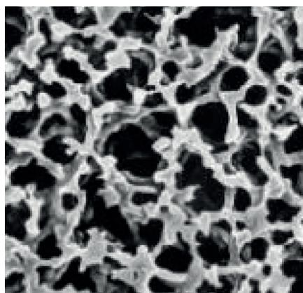
Figure 2: Scanning electron micrograph of a Millipore membrane filter (pore size 0.22 µm) showing a distribution of pore sizes.<sup>10</sup> (Bar in bottom right hand corner of image is 1 µm long.)
