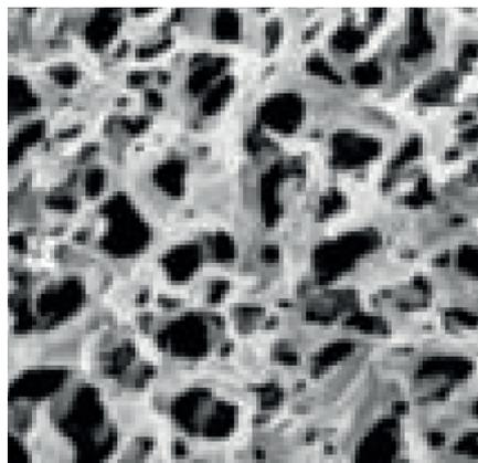
Figure 1: Scanning electron micrograph of nylon membrane filter (pore size 0.22 µm).
