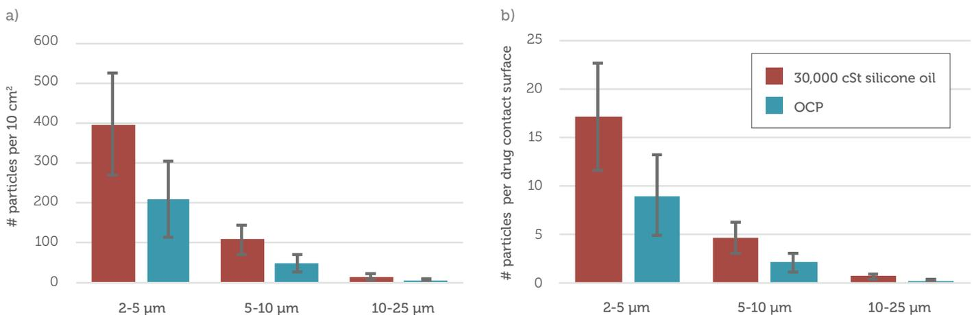
Figure 6: Subvisible particle loads for uncoated, siliconised (30,000 cSt) bromobutyl plungers (red) and OmniflexCP® (blue) (a) normalised to 10 cm² of rubber and (b) per drug contact surface area.
