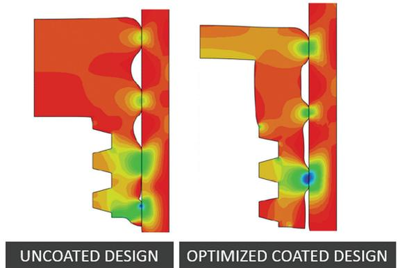
Figure 2: FEA simulations of the compressive stress profiles of the 1-3 mL uncoated (left) and OmniflexCP® (right) plunger designs.
