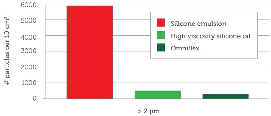
Figure 5: Number of SbVP's (>2µm) per 10 cm² measured according to ISO 8871-3 for a bromobutyl closure siliconised with 350 cSt silicone oil (red), 30,000 cSt silicone oil (light green), and Omniflex coated (dark green).
