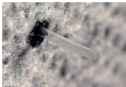
**Figure 3: Automatic needle insertion system with soft cannula remaining in the body after insertion.**
