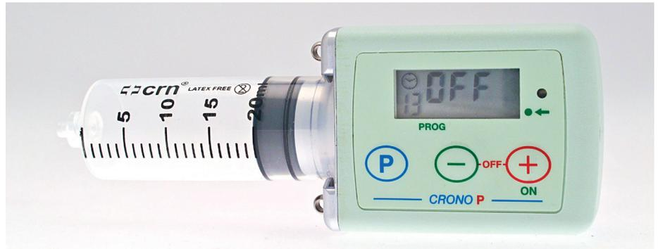
Figure 4: The Crono P is a pump for the infusion of hormones following the body's natural rhythms. The infusion takes the form of a series of boluses at intervals of either 90 or 180 minutes, with a volume which may be programmed from 5  $\mu$ L to 1000  $\mu$ L. The day can be divided into up to three periods, with a different bolus volume programmed for each, such that the circadian and ultradian cycles may be reproduced as required.
