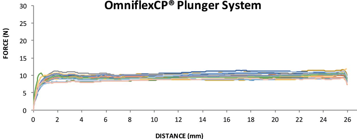
Figure 7: Extrusion forces for the Gx Baked-on RTF® / OmniflexCP® syringe system. The 1 mL, long staked needle syringes (27G) were WFI filled. Plungers were steam sterilised and placed by vacuum placement. The system was aged for one year. Twenty syringe samples were measured at a displacement rate of 380 mm/min..
