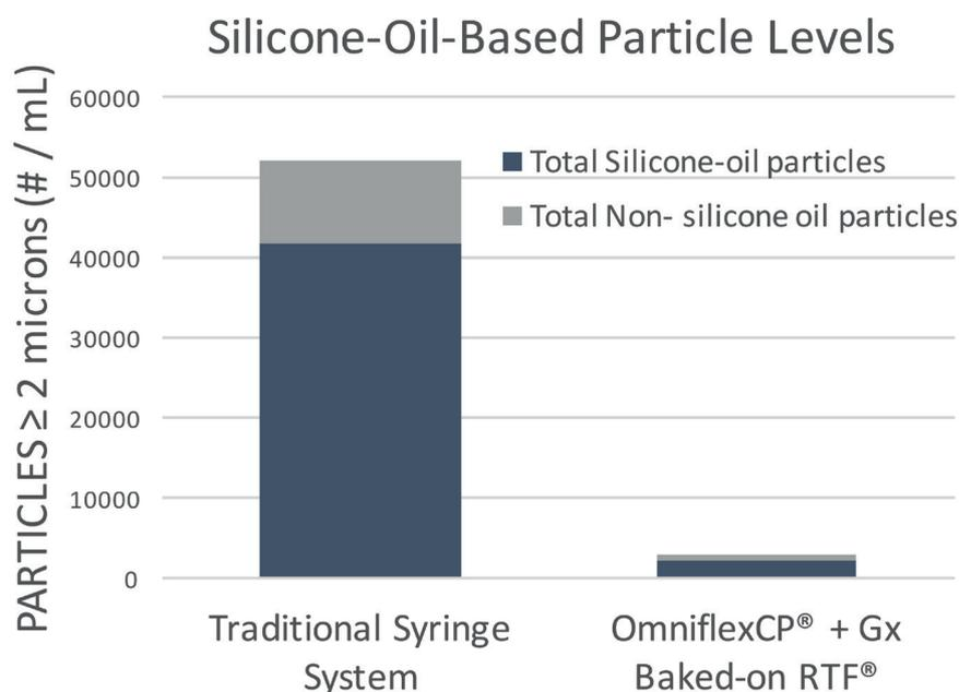
Figure 6: Particle level measurements by MFI in a traditional syringe system (left bar, free silicone on the barrel and a high viscosity siliconised plunger) versus the Gx Baked-on RTF® Syringe with OmniflexCP® (right). Syringes have been aged under accelerated conditions for three months. The blue portion of the bars represent silicone-oil-based particles and the grey portion of the bars represent other particles.
