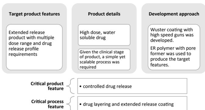
Figure 6: Scheme for development of extended release pellets.
