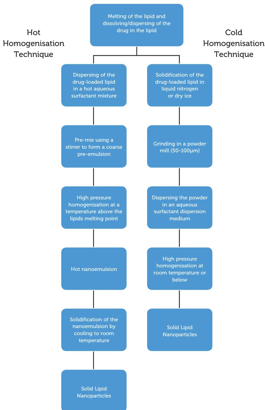
Figure 4: Schematic of SLN production by hot and cold HPH.<sup>6</sup>
