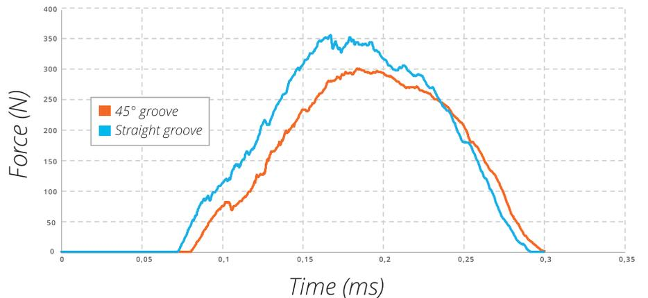
Figure 7: Shock force (N) on the syringe / syringe housing during the simulated autoinjection.
