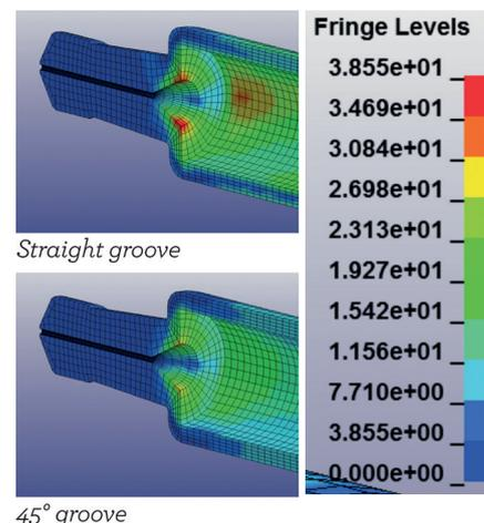
Figure 9: Simulated stress maps of the two autoinjector designs (top) straight cam and (bottom) 45° cam.
