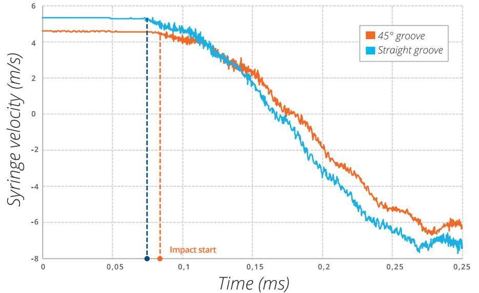
Figure 5: Syringe velocity (m/s) over time during simulation auto-injections using a 45° orientated cam and a straight cam design.
