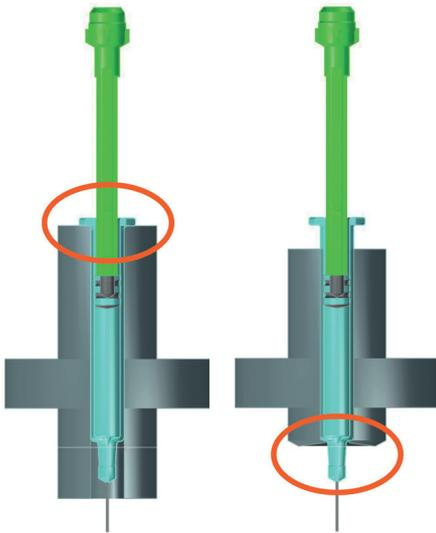
Figure 4: Gripping syringe on the shoulders (right) instead of the flange (left) reduces overall stress.
