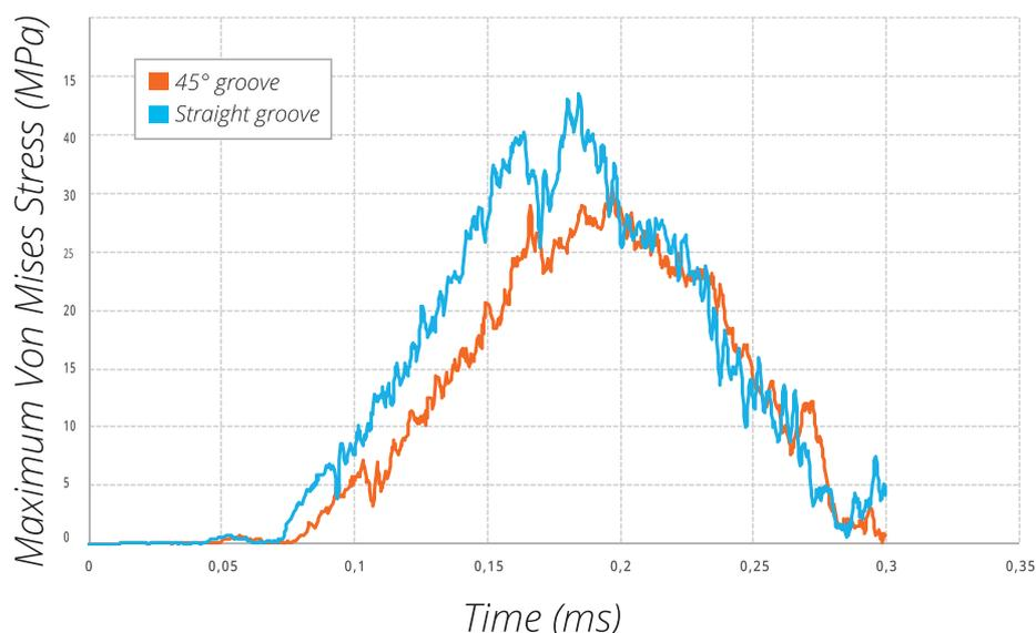
Figure 8: Maximum stress (MPa) on the syringe from the simulated autoinjection with 45° cam compared with straight cam.
