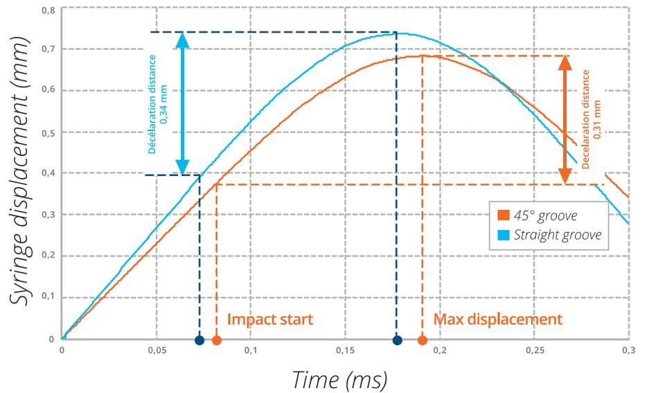
Figure 6: Syringe displacement distances (mm) over the course of the simulated autoinjection.
