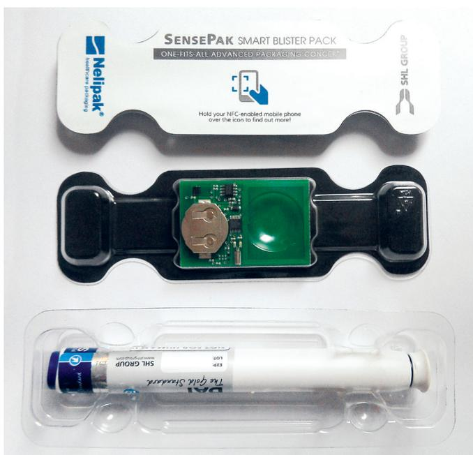
Figure 6: SensePak smart packaging under development with SHL Group. (Image courtesy SHL Group)
