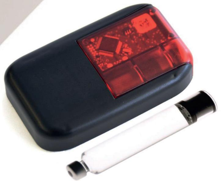
Designed to accept standard 3 ml insulin cartridges, yet barely larger than the cartridge itself, the system is extremely small and still incorporates all functions needed.
