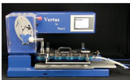
Figure 1: The Vertus can be used with a wide range of collection devices including NGI (shown here), ACI, DUSAs and waste filters.
