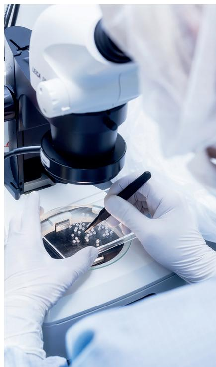
Figure 4: AQL inspection of micro parts in a Class 7 cleanroom environment.
