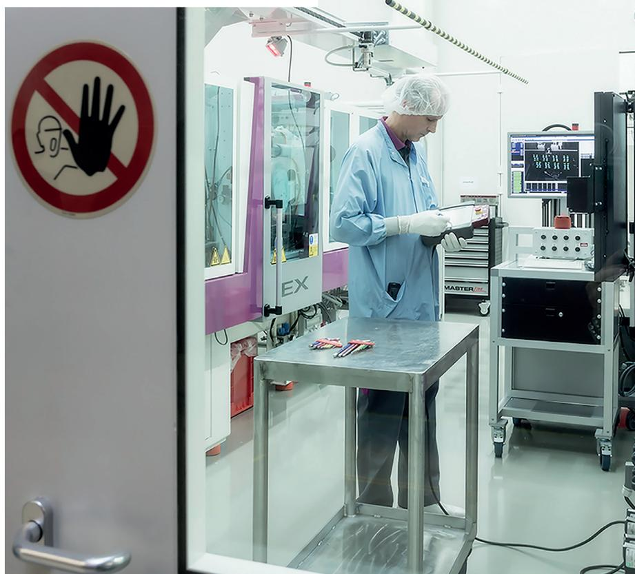
Figure 2: One of Trelleborg's Class 8 cleanrooms where safety-critical medical LSR components are produced fully automatically to a zero-defect policy.
