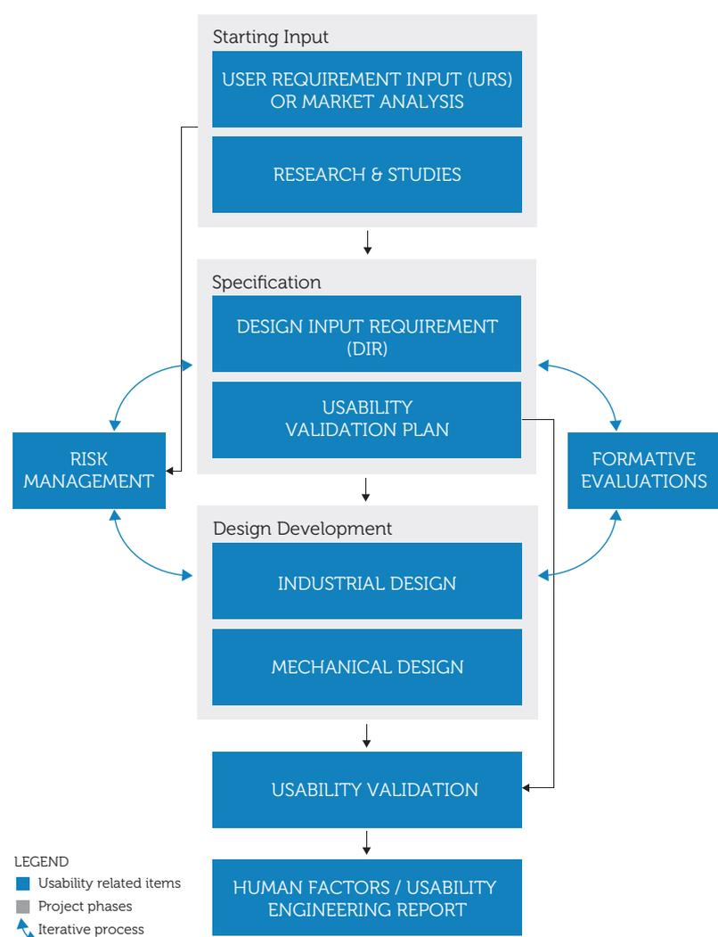
Figure 3: A simplified functionality usability flowchart for the design and development of auto injectors.
