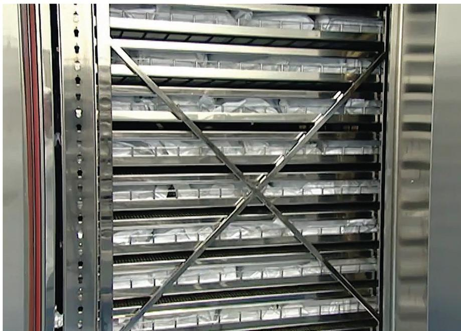
Figure 3: The autoclave used in steam sterilisation is equipped with an external jacket aimed to stabilise the conditions of temperature and pressure inside it across the entire sterilisation cycle. Saturated water vapour is blown inside.
