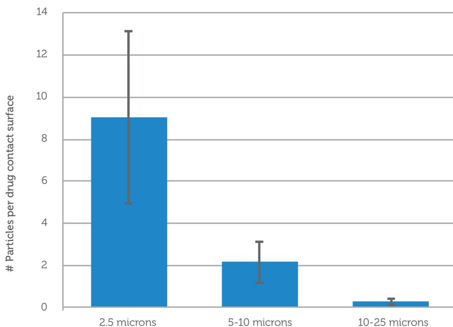
Figure 3: Number of particles per drug contact surface area of a 1 mL long syringe plunger for OmniflexCP<sup>®</sup>. Particle counts are determined in accordance with the method outlined in ISO 8871-3.
