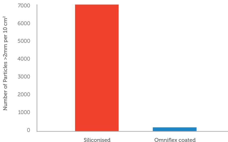
Figure 2: Number of particles greater than 2  $\mu\text{m}$  in size, normalised to 10  $\text{cm}^2$  of rubber, for elastomeric closures that have been siliconised with a low viscosity (350 cSt) silicone oil (red bar) versus elastomeric closures that have been Omniflex coated (blue bar). Particle counts are determined in accordance with the method outlined in ISO 8871-3.
