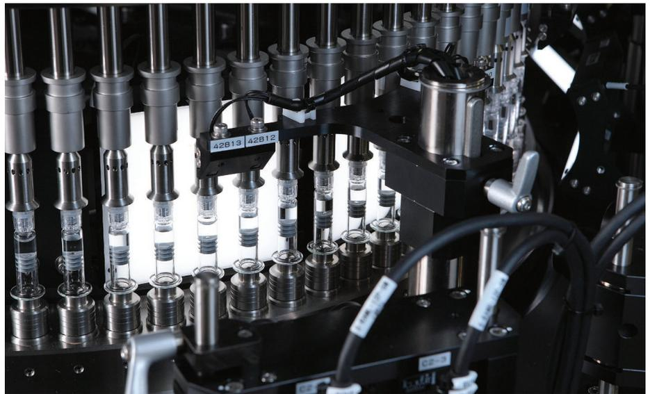
Figure 2: Inspection system with LED lighting.
