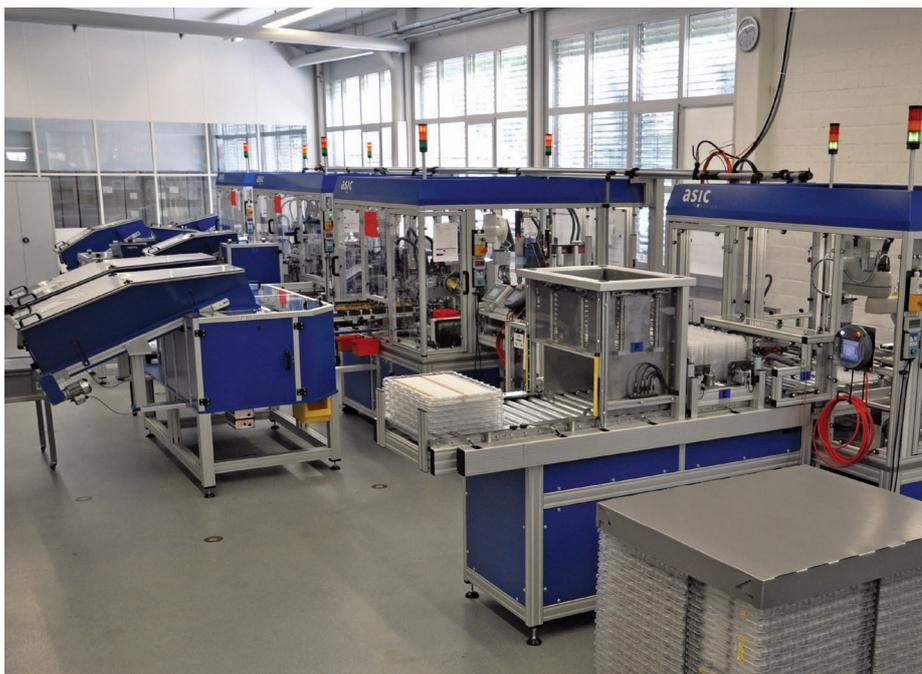
Figure 4: Flexible assembly line for fully customised YpsoMate® auto injectors at one of Ypsomed's Swiss manufacturing sites.
