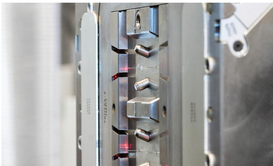
Figure 3: Cannula mounted in b-side of injection mould.
