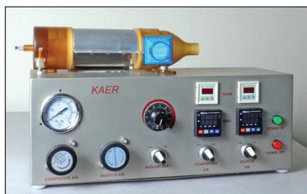
**Figure 3: Preclinical version of SUPRAER with the requisite controls to enable the optimisation of the airflows and heating parameters for each API.**
