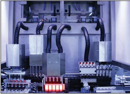
**Figure 2: Mikron G05 for Pharma/Medical application – Easy cleaning due to physical separation of the assembly area, covered process and handling stations.**
