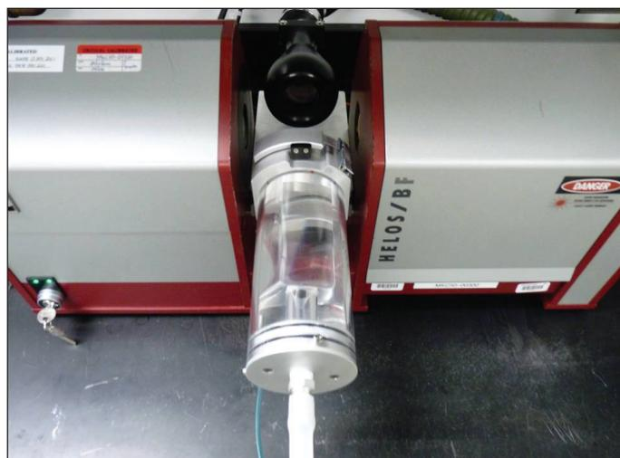
**Figure 5. Laser diffraction instrument shown with MannKind's inhaler module.**
